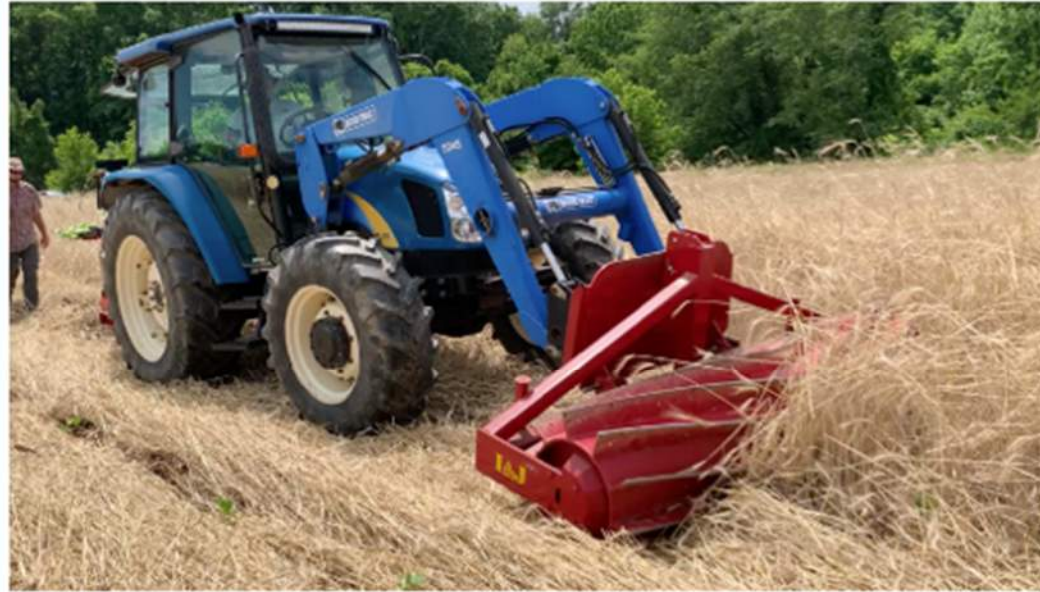
Roller-crimper rolls down the terminated cereal crop cover crop ahead of transplanting. The cover crop residue reduces runoff, increases water infiltration, suppresses weeds, and adds organic matter to soils.
